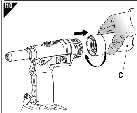
To assemble the baffle (T) proceed as follows: remove the nail tank (C) (pic. F10) as well as the cover (R), assemble the reduction (S) on the connector and insert the baffle (T) with a slight pressure.
