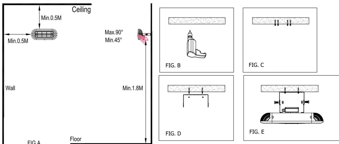
**ATTENTION:** The heater has to be fixed on walls, where there are no combustible materials positioned, directly above the appliance or in any case in the immediate vicinity. Otherwise, place the product at a minimum distance of 1 m from the ceiling, from the lateral walls and from other thermo-sensitive materials.
