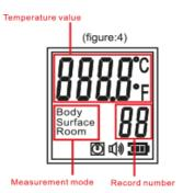
Under the mode of viewing temperature records, when the storage icon flashes, MEM key can be pressed for ON/ OFF of voice symbol. (Common edition has no this function).
